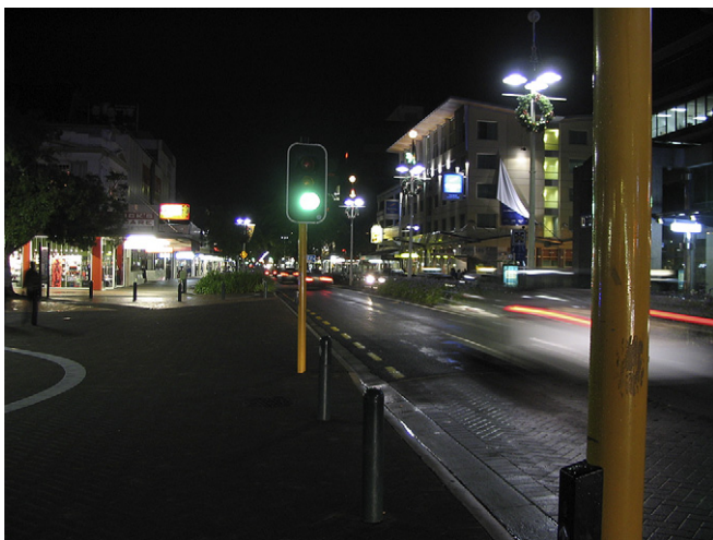
Fig. 2. A typical town night scene. The lowest luminance is on the ground and on the street where it should be about 1 \text{ cd/m}^2 . Its luminance is even lower than the night sky in big cities. Most of the rest of the scene has a far higher luminance, completely in the photopic range of our eyes. (Photo by Bruce Kingsbury).
